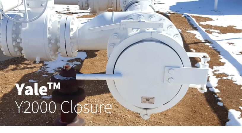
Our Yale Y2000 is a clamp-style closure that is designed specifically for pipeline application, currently 6" to 24". The operation is simple, safe, does not require special tools and does not require the operator to place himself in harm's way during any step of the opening process. Our standard design codes were designed to meet ASME BPVC Sec. VIII, Div.1 Our Y2000 is the perfect alternative to the traditional threaded closure.
